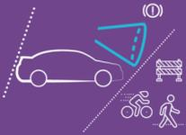
**Advanced emergency braking systems:** recognising obstacles (pedestrians, cyclists, other vehicles...) and applying pressure on the brakes in order to prevent a collision.
