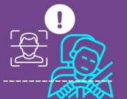
**Drowsiness and awareness monitoring:** detecting whether the driver is falling asleep (e.g. drooping eyelids, blink rate) or distracted (e.g. face turned towards a passenger or phone), using interior cameras and sensors, in order to issue a warning and apply an appropriate intervention.
