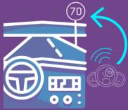
**Intelligent speed adaptation:** detecting and identifying speed limits from traffic signs and displaying these on the dashboard, or even automatically adjusting the vehicle's speed.
